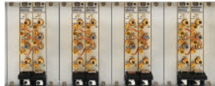
▲ Fig. 5 This multi-site configuration example includes a quartet of independent four-port PXI VNAs in a single chassis.
