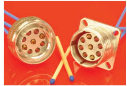
▲ Fig. 3 TQ-9 Multiport: 9 × 40 GHz coaxial cable assemblies in the MIL-DTL-38999, size 13.
