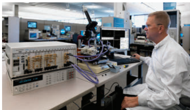
▲ Fig. 2 Adding a pair of two-port PXI VNAs to an existing test station enables powerful device characterization without expanding system height or footprint.
