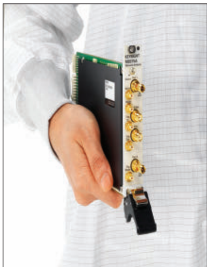
▲ Fig. 1 A new class of PXI VNAs offers full two-port capability—including a source—in a single slot.
